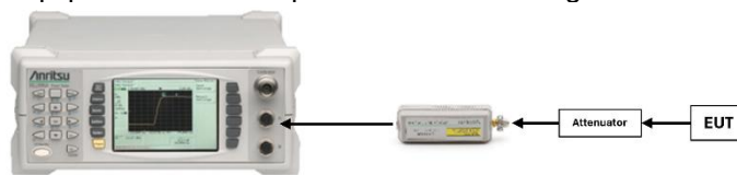
Figure 7-3. Test Instrument & Measurement Setup for Power Meter Measurements
