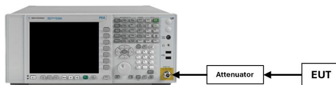
Figure 7-5. Test Instrument & Measurement Setup
