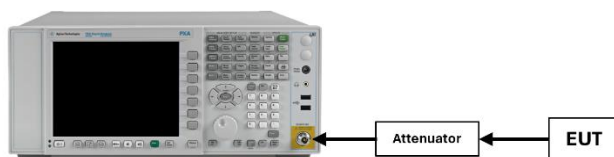
Figure 7-1. Test Instrument & Measurement Setup
