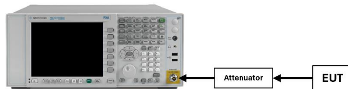
Figure 7-5. Test Instrument & Measurement Setup
