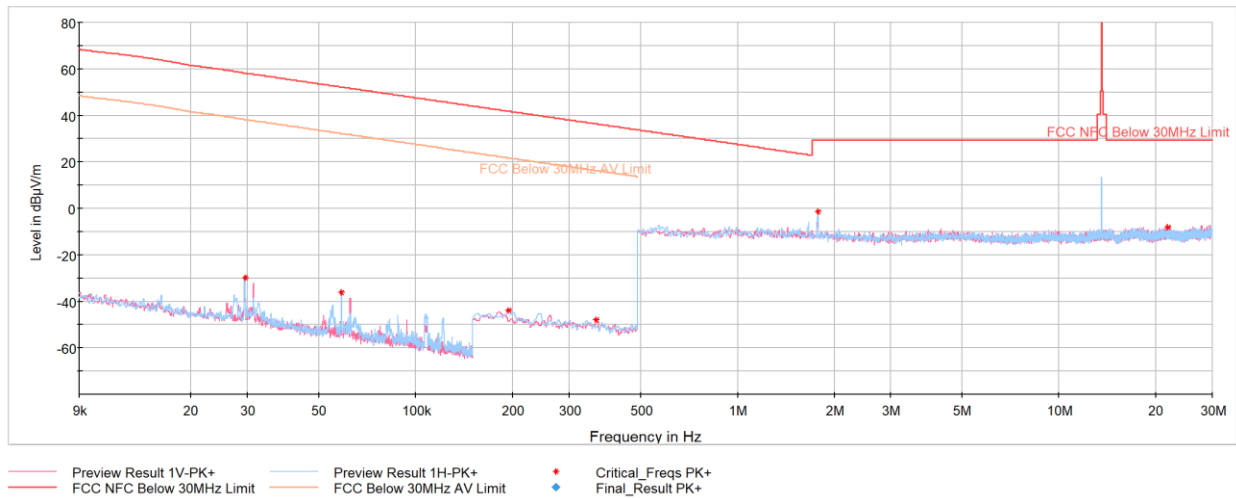
Plot 7-8. Radiated Spurious Emissions 9kHz – 30MHz (CE F 424kbps, with AC/DC Adapter and Magnetic Charger)
