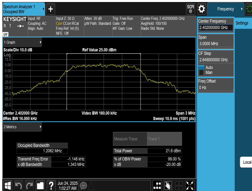
Plot 7-4. 20dB BW and 99% OBW Plot (Bluetooth, 8DPSK, ePA – Ch. 0)
