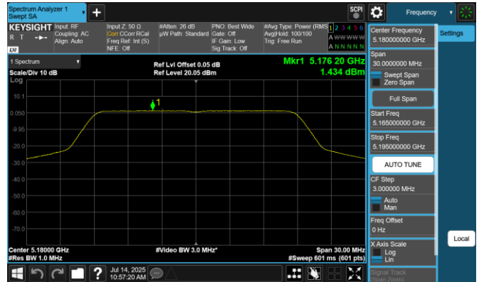
Plot 7-16. ISD PSD (20MHz BW 802.11n - Ch. 36, MCS0)
