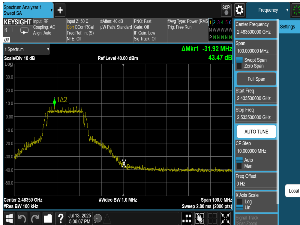
Plot 7-31. Band Edge Plot (802.11g – Ch. 10) – 6Mbps
