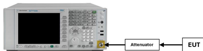
Figure 7-3. Test Instrument & Measurement Setup
