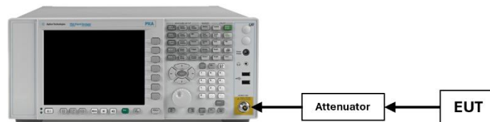
Figure 7-3. Test Instrument & Measurement Setup
