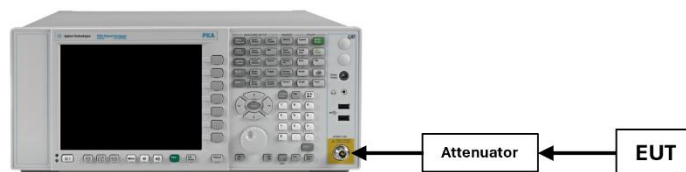
Figure 7-3. Test Instrument & Measurement Setup
