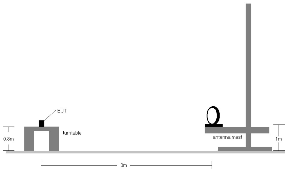
Figure 7-6. Radiated Test Setup < 30MHz
