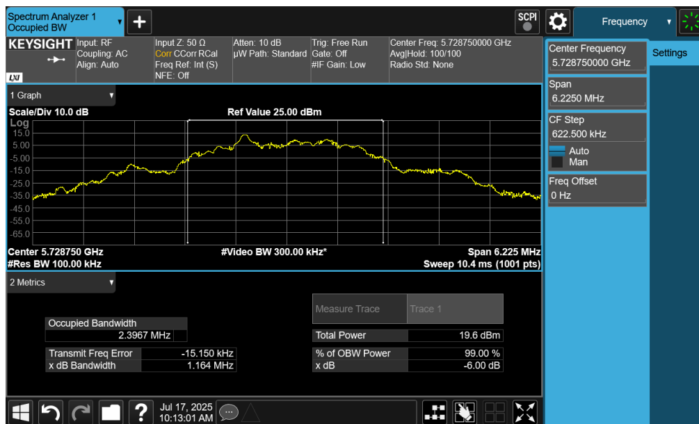
Plot 7-4. 6dB BW & 99% OBW (O-QPSK, 5728.75MHz, 500kpbs)
