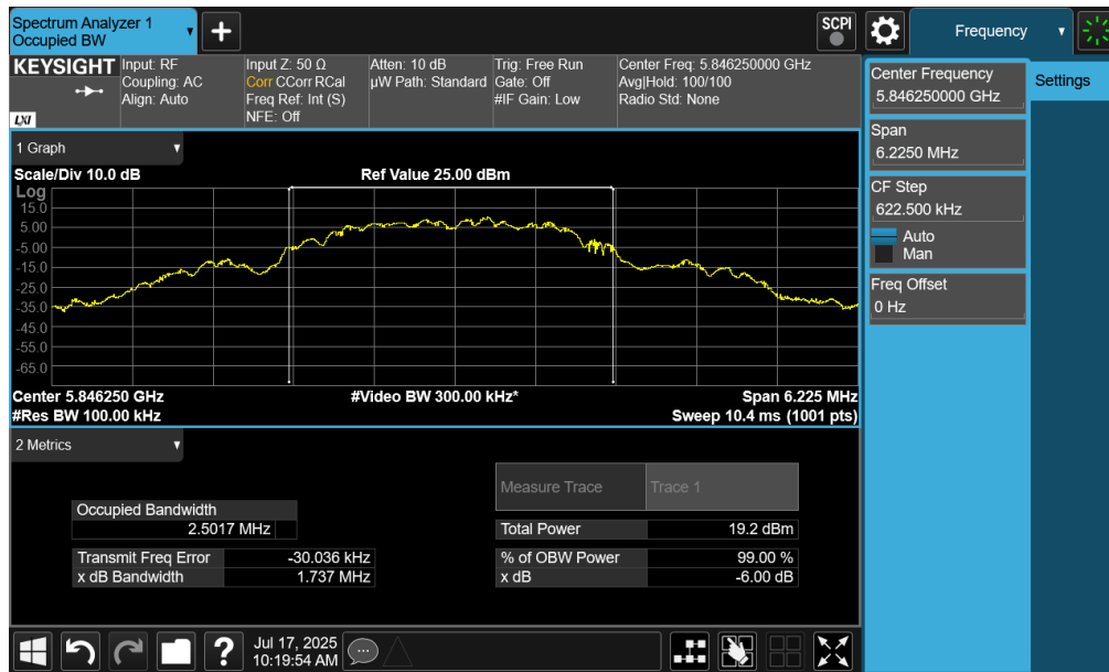
Plot 7-3. 6dB BW & 99% OBW (O-QPSK, 5846.25MHz, 250kpbs)
