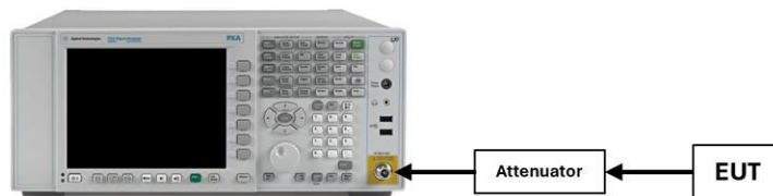
Figure 7-1. Test Instrument & Measurement Setup
