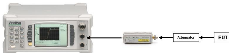
Figure 7-3. Test Instrument & Measurement Setup
