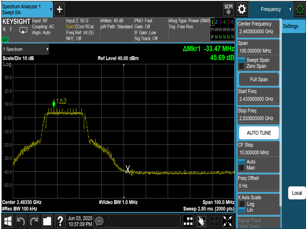
Plot 7-30. Band Edge Plot (802.11g – Ch. 10) – 6Mbps
