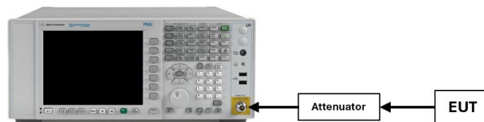
Figure 7-1. Test Instrument & Measurement Setup
