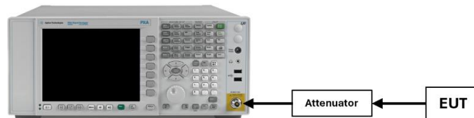
Figure 7-3. Test Instrument & Measurement Setup
