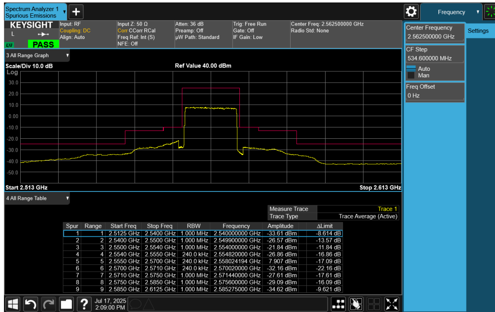
Plot 7-92. Upper ACP Plot (LTE Band 7 - 15MHz QPSK - Full RB)
