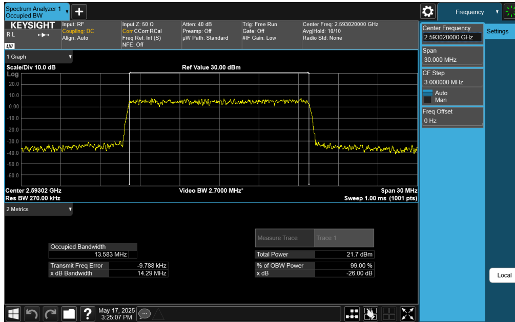
Plot 7-39. Occupied Bandwidth Plot (NR Band n41 - 15MHz CP-OFDM 16-QAM - Full RB)
