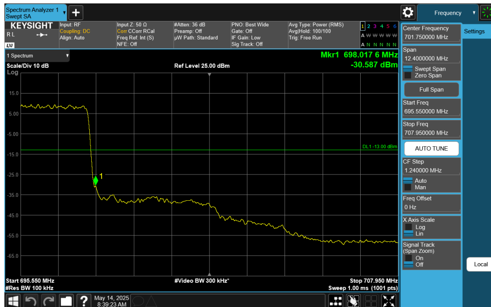
Plot 7-229. Upper Band Edge Plot (NR Band n71 – 5.0MHz DFT-s-OFDM \pi/2 BPSK - Full RB)
