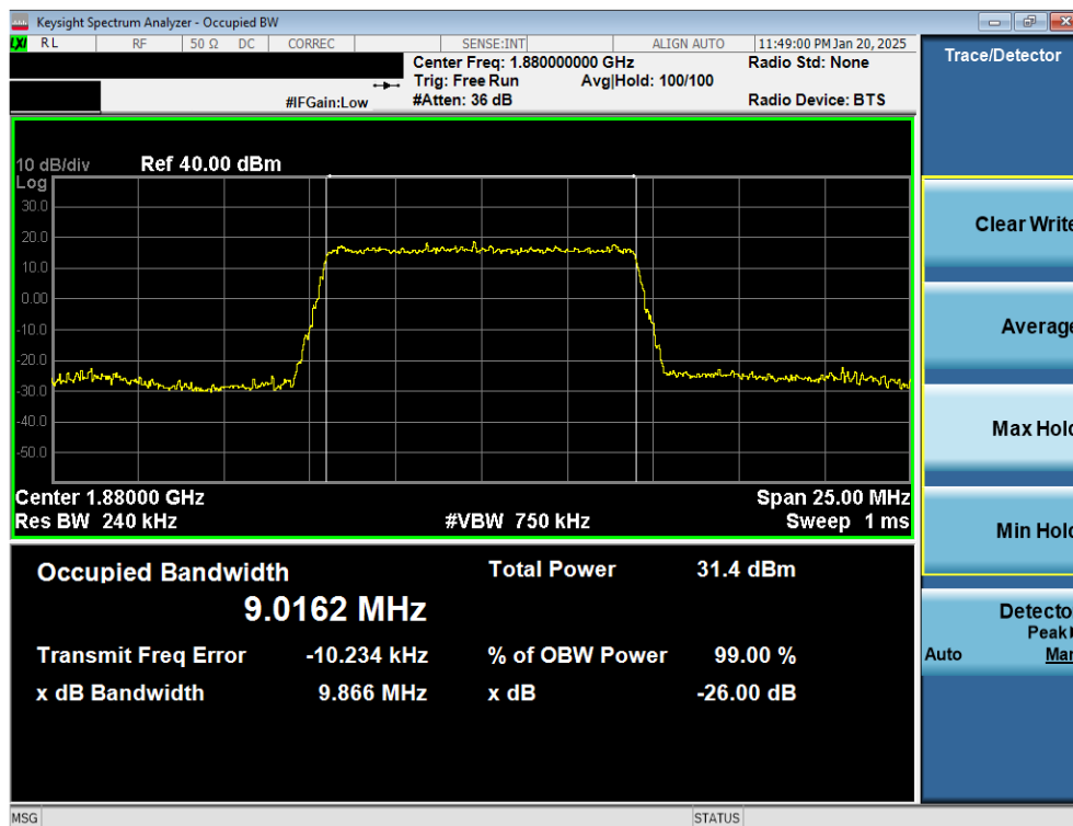
Plot 7-7. Occupied Bandwidth Plot (LTE Band 25/2 - 10MHz QPSK - Full RB Configuration)
