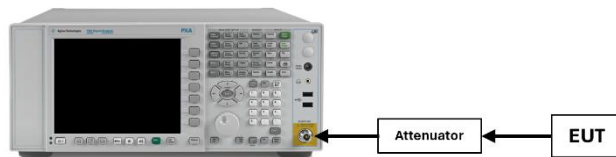
Figure 7-5. Test Instrument & Measurement Setup
