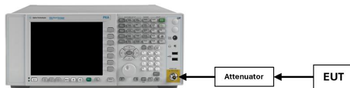
Figure 7-7. Test Instrument & Measurement Setup
