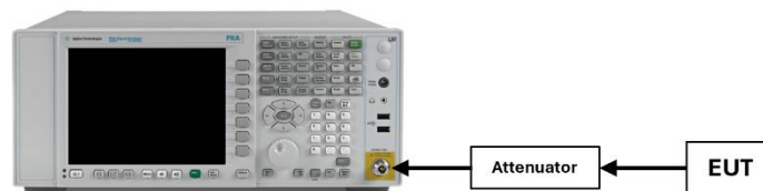
Figure 7-3. Test Instrument & Measurement Setup
