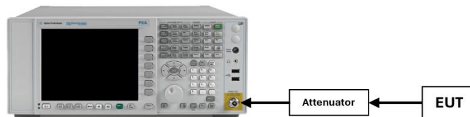
Figure 7-4. Test Instrument & Measurement Setup
