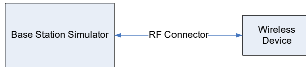
Figure 8-1 Power Measurement Setup
