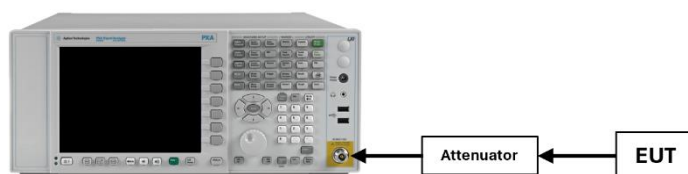
Figure 7-3. Test Instrument & Measurement Setup
