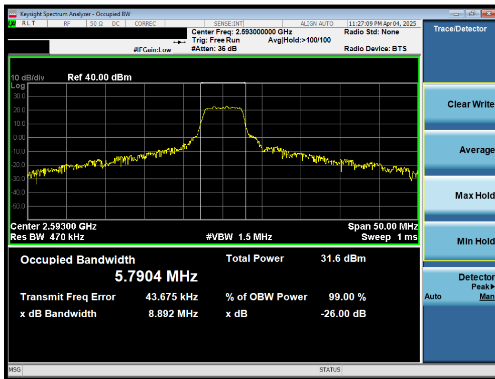
Plot 7-16. Occupied Bandwidth Plot (LTE Band 41 - 20MHz 16-QAM - Full RB)
