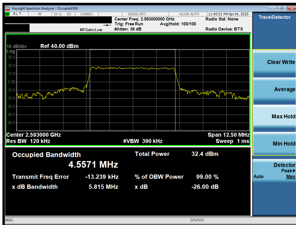
Plot 7-9. Occupied Bandwidth Plot (LTE Band 41 - 5MHz QPSK - Full RB)
