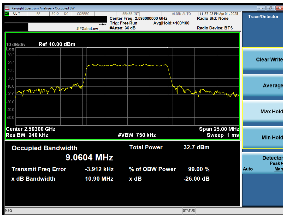
Plot 7-11. Occupied Bandwidth Plot (LTE Band 41 - 10MHz QPSK - Full RB)
