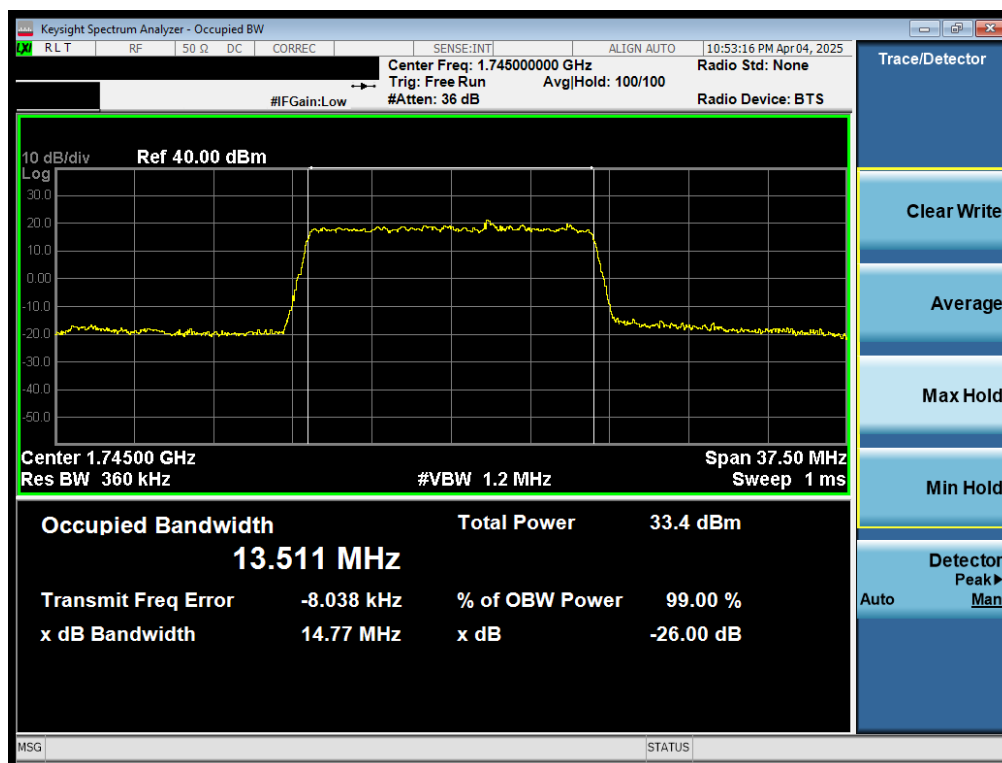
Plot 7-9. Occupied Bandwidth Plot (LTE Band 66/4 - 15MHz QPSK - Full RB)
