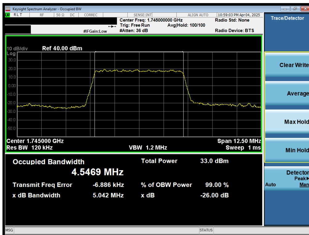
Plot 7-5. Occupied Bandwidth Plot (LTE Band 66/4 - 5MHz QPSK - Full RB)
