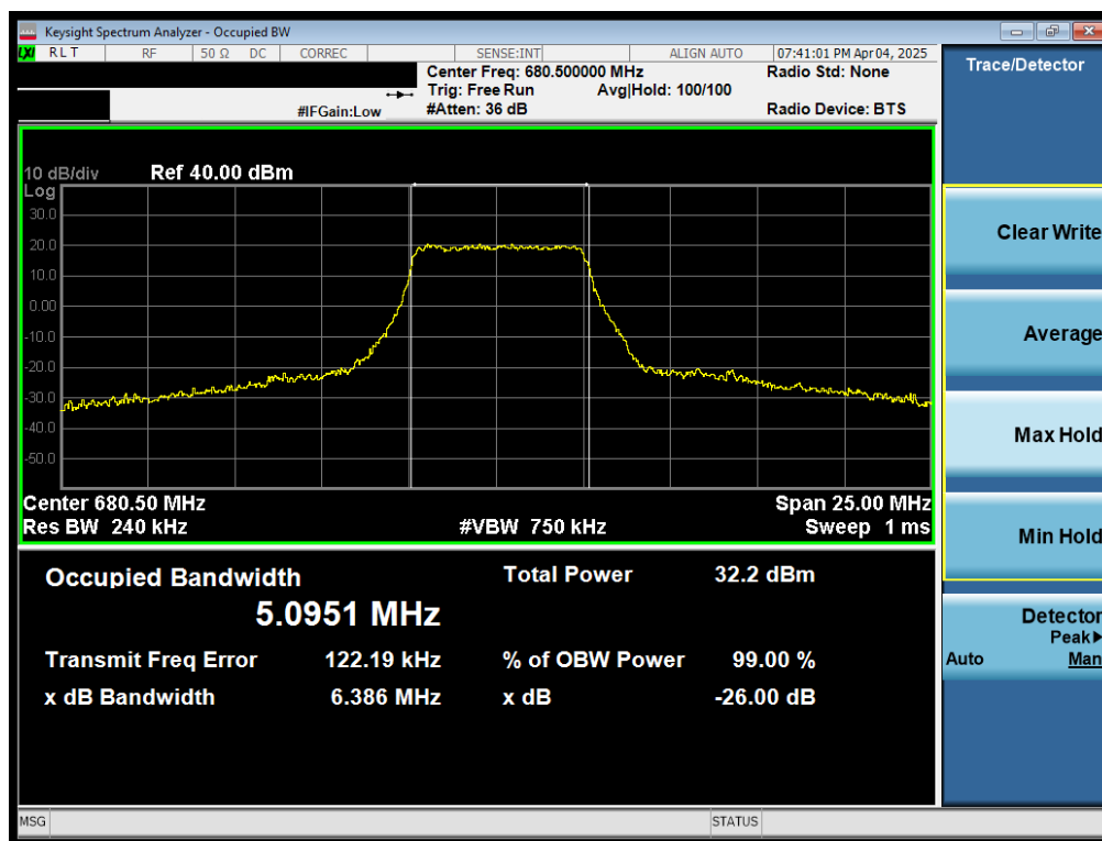
Plot 7-16. Occupied Bandwidth Plot (LTE Band 71 - 10MHz 16-QAM - Full RB)
