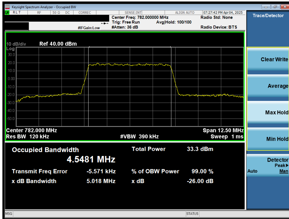
Plot 7-29. Occupied Bandwidth Plot (LTE Band 13 - 5MHz QPSK - Full RB)
