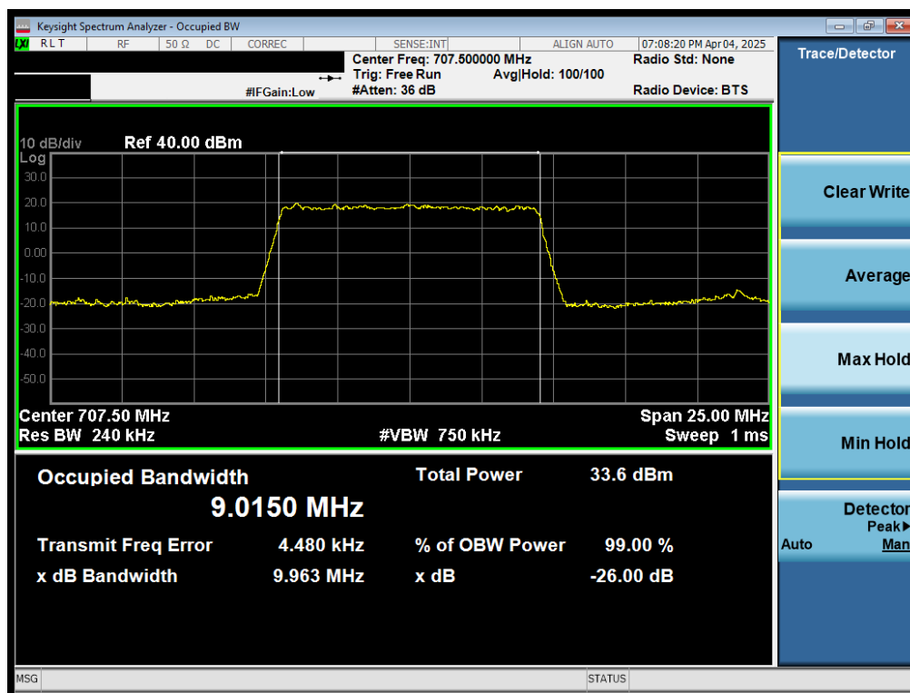
Plot 7-27. Occupied Bandwidth Plot (LTE Band 12/17 - 10MHz QPSK - Full RB)
