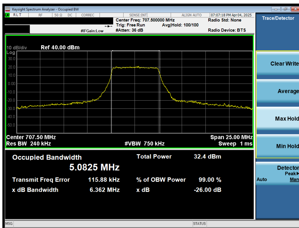
Plot 7-28. Occupied Bandwidth Plot (LTE Band 12/17 - 10MHz 16-QAM - Full RB)
