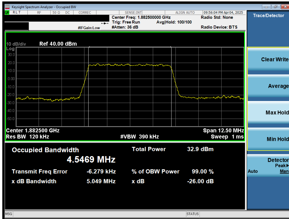
Plot 7-5. Occupied Bandwidth Plot (LTE Band 25/2 - 5MHz QPSK - Full RB Configuration)
