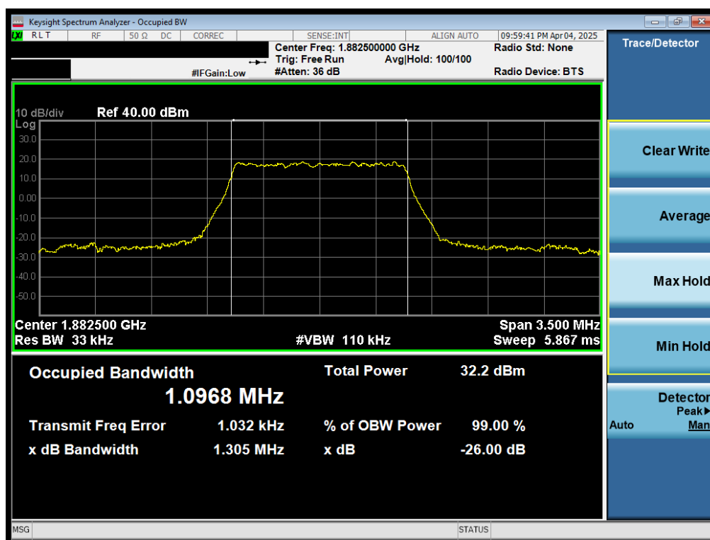
Plot 7-1. Occupied Bandwidth Plot (LTE Band 25/2 - 1.4MHz QPSK - Full RB Configuration)
