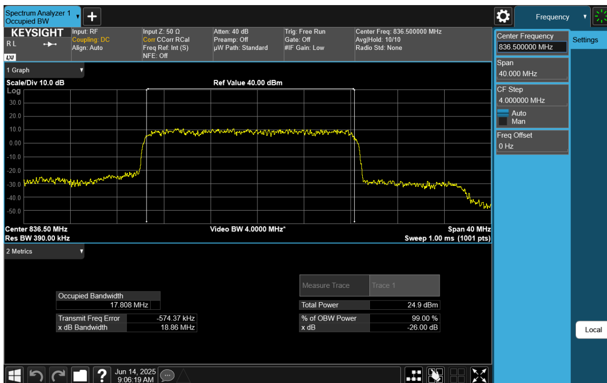
Plot 7-21. Occupied Bandwidth Plot (NR Band n26/n5 - 20MHz DFT-s-OFDM \pi/2 BPSK - Full RB Configuration)
