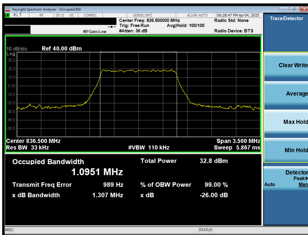
Plot 7-1. Occupied Bandwidth Plot (LTE Band 26/5 - 1.4MHz QPSK - Full RB Configuration)
