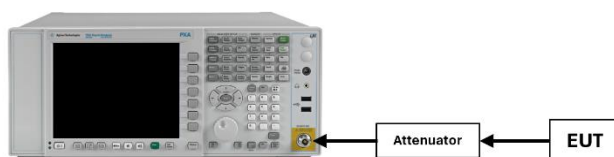
Figure 7-3. Test Instrument & Measurement Setup
