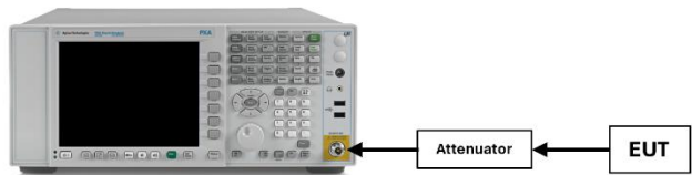
Figure 7-1. Test Instrument & Measurement Setup
