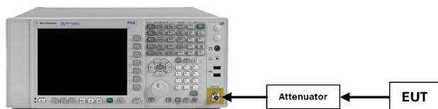
Figure 7-5. Test Instrument & Measurement Setup
