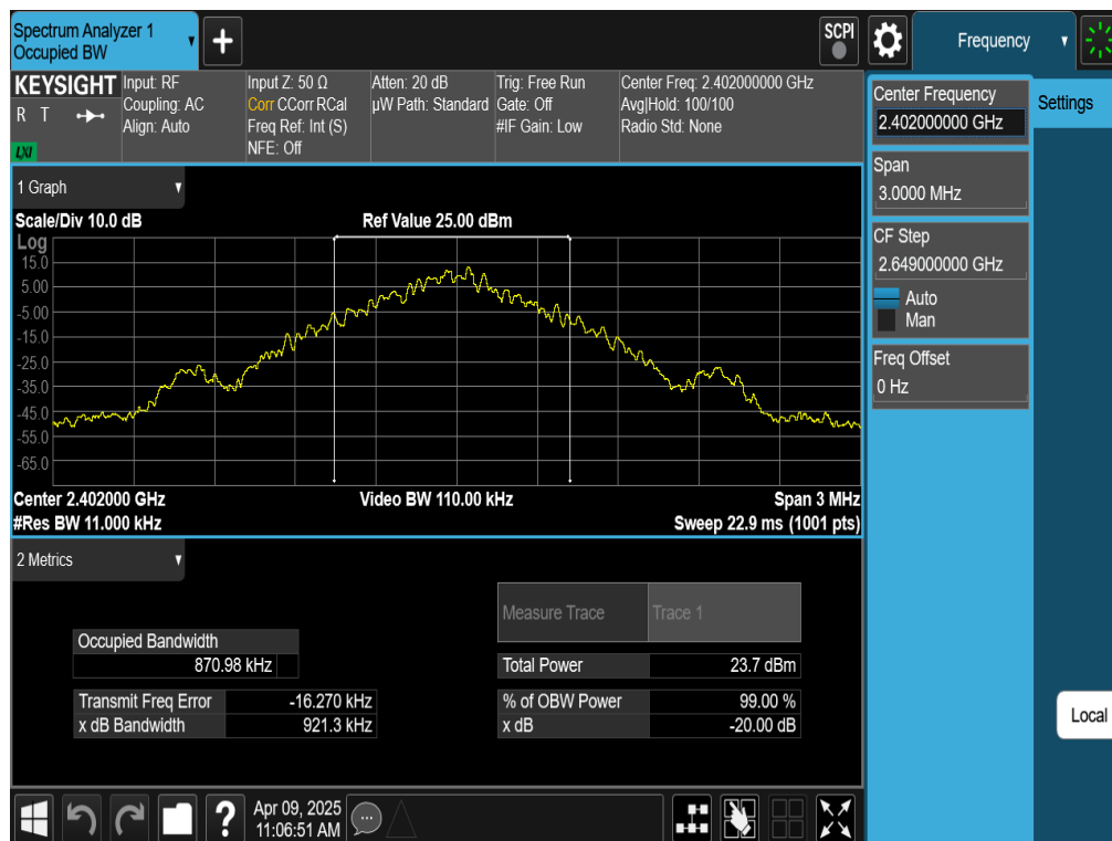
Plot 7-1. 20dB BW and 99% OBW Plot (Bluetooth, GFSK, ePA – Ch. 0)
