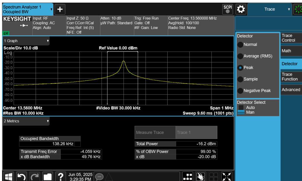
Plot 7-1. 20dB and 99% Bandwidth Plot (CE A 106kbps)
