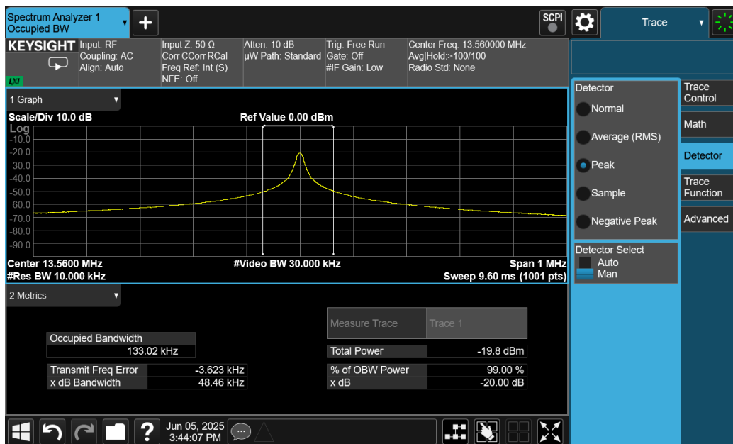
Plot 7-2. 20dB and 99% Bandwidth Plot (CE B 106kbps)
