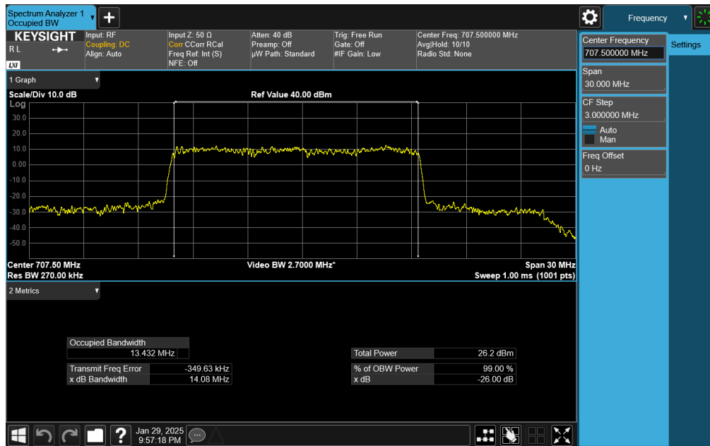
Plot 7-73. Occupied Bandwidth Plot (NR Band n12 - 15MHz DFT-s-OFDM \pi/2 BPSK - Full RB)
