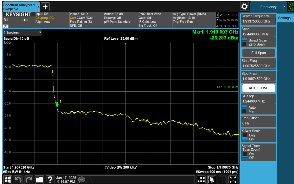
Plot 7-113. Upper Band Edge Plot (NR Band n2 – 5MHz DFT-s-OFDM \pi/2 BPSK – Full RB Configuration)
