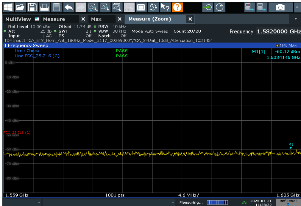
Plot 7-26. Radiated Spurious Plot – (1559 – 1610MHz) – Low Channel – Vertical
