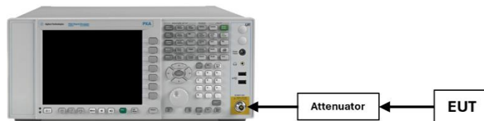
Figure 7-4. Test Instrument & Measurement Setup
