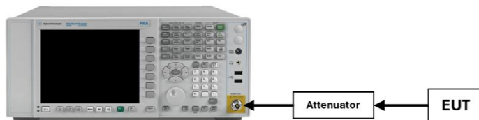
Figure 7-2. Test Instrument & Measurement Setup
