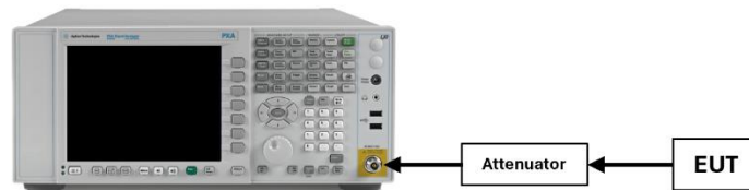
Figure 7-3. Test Instrument & Measurement Setup
