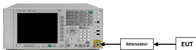
Figure 7-1. Test Instrument & Measurement Setup
