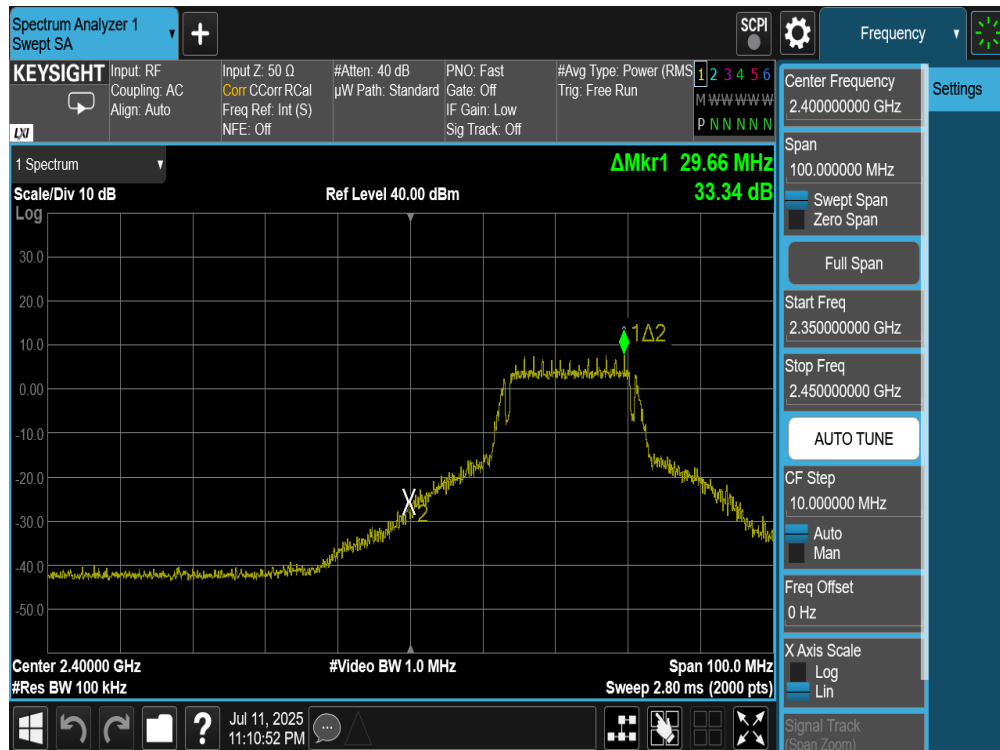
Plot 7-31. Band Edge Plot (802.11g– Ch. 3) – 6Mbps
