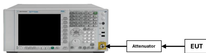
Figure 7-4. Test Instrument & Measurement Setup
