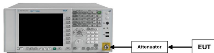
Figure 7-3. Test Instrument & Measurement Setup
