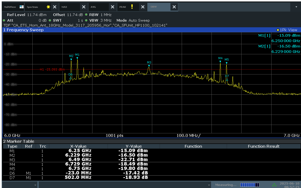
Plot 7-1. 10dBc Bandwidth (Ch. 5, Config 9/Payload 65B)
