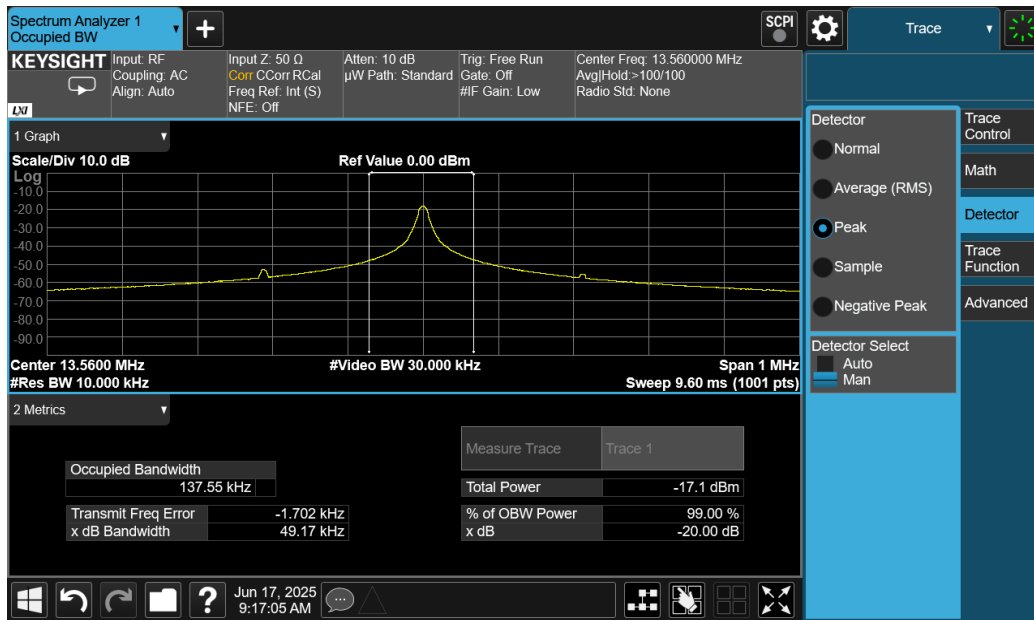
Plot 7-3. 20dB and 99% Bandwidth Plot (CE F 212kbps)
