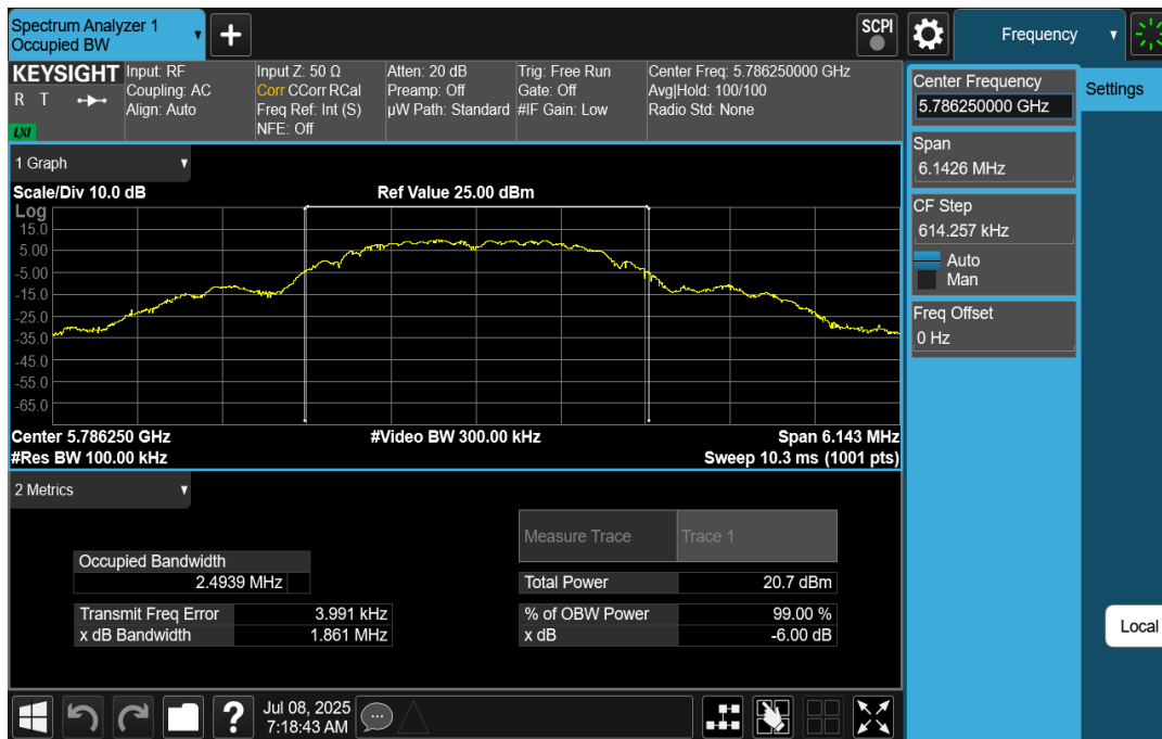
Plot 7-2. 6dB BW & 99% OBW (O-QPSK – 5786.25MHz, 250kbps)
