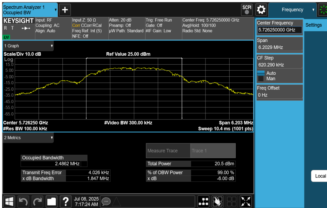
Plot 7-1. 6dB BW & 99% OBW (O-QPSK – 5726.25MHz, 250kbps)
