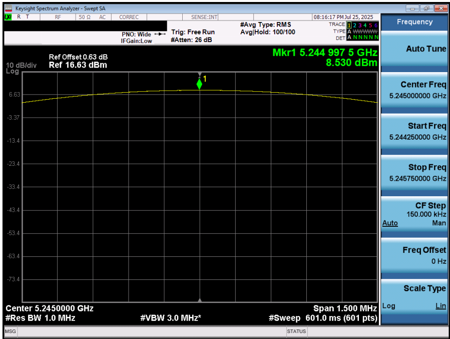
Plot 7-48. PSD (NB UNII LE1M – 5245MHz)
