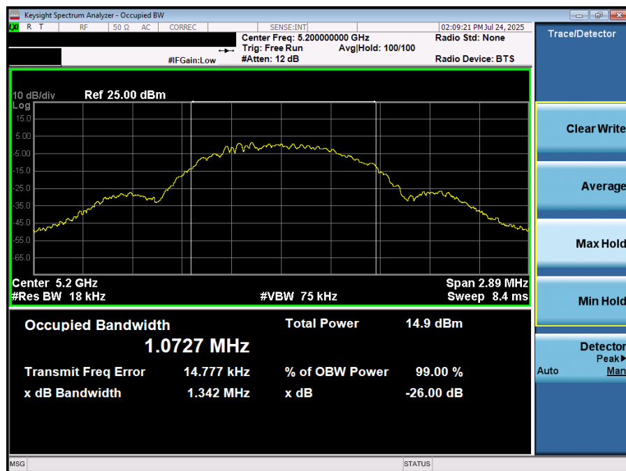
Plot 7-5. 26dB BW & 99% OBW (NB UNII LE1M – 5200MHz)
