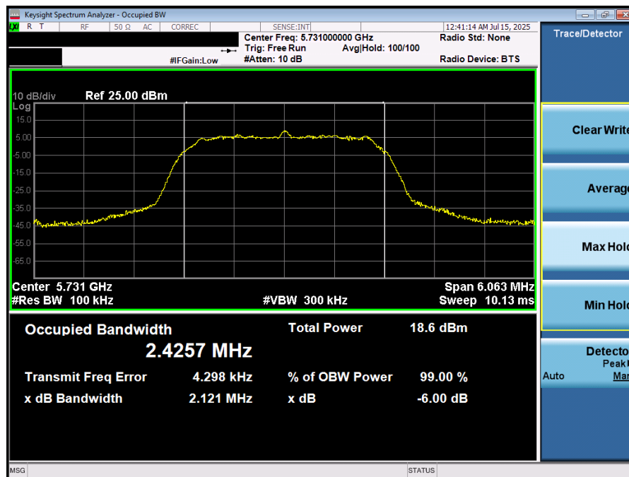
Plot 7-37. 6dB BW & 99% OBW (NB UNII HDRp4 – 5731MHz)
