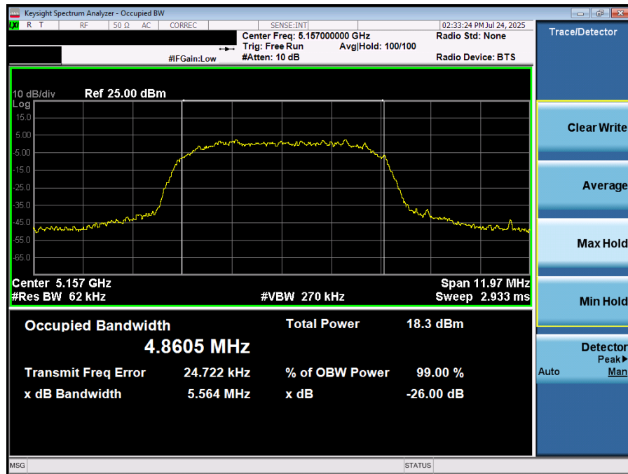
Plot 7-19. 26dB BW & 99% OBW (NB UNII HDRp8- 5157MHz)
