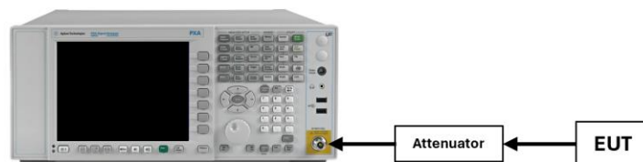
Figure 7-1. Test Instrument & Measurement Setup
