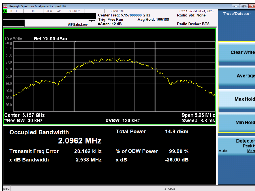
Plot 7-7. 26dB BW & 99% OBW (NB UNII LE2M – 5157MHz)
