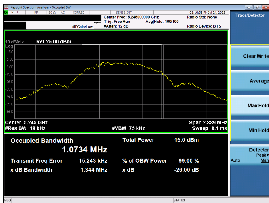
Plot 7-6. 26dB BW & 99% OBW (NB UNII LE1M – 5245MHz)
