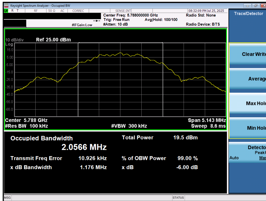
Plot 7-29. 6dB BW & 99% OBW (NB UNII LE2M – 5788MHz)
