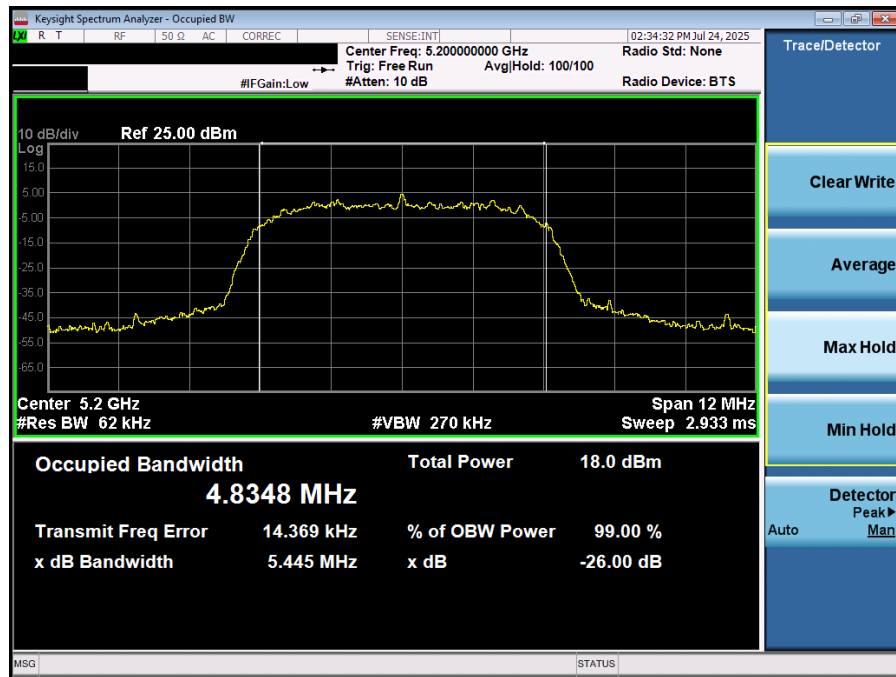
Plot 7-20. 26dB BW & 99% OBW (NB UNII HDRp8- 5200MHz)
