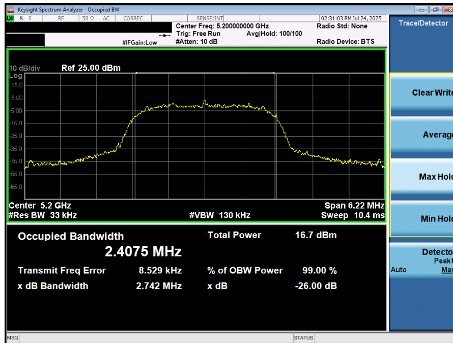
Plot 7-17. 26dB BW & 99% OBW (NB UNII HDRp4- 5200MHz)
