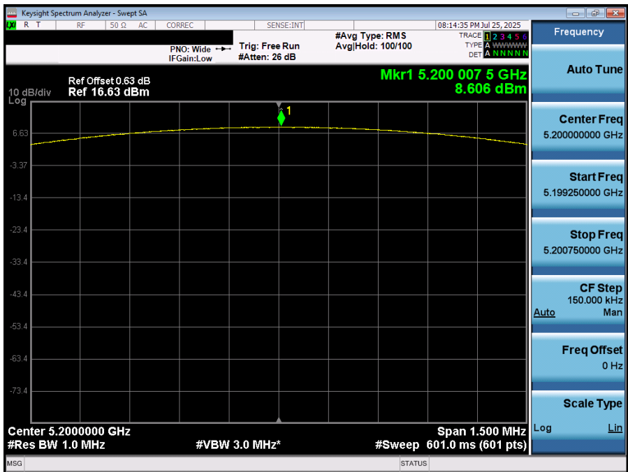
Plot 7-47. PSD (NB UNII LE1M – 5200MHz)
