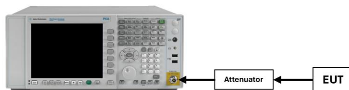
Figure 7-4. Test Instrument & Measurement Setup
