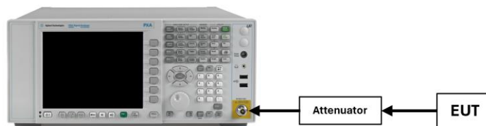
Figure 7-3. Test Instrument & Measurement Setup
