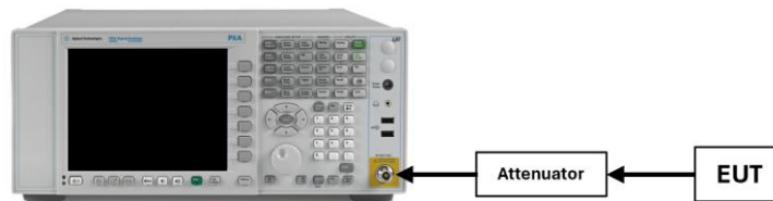
Figure 7-7. Test Instrument & Measurement Setup
