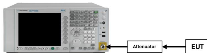
Figure 7-4. Test Instrument & Measurement Setup
