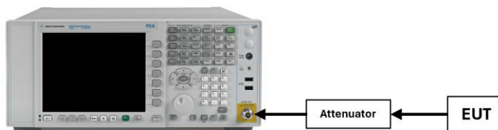
Figure 7-1. Test Instrument & Measurement Setup
