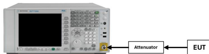
Figure 7-5. Test Instrument & Measurement Setup
