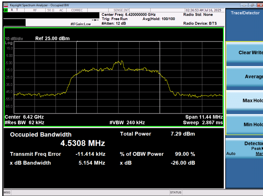
Plot 7-15. 26dB BW & 99% OBW (NB UNII HDR8 – 6420MHz)
