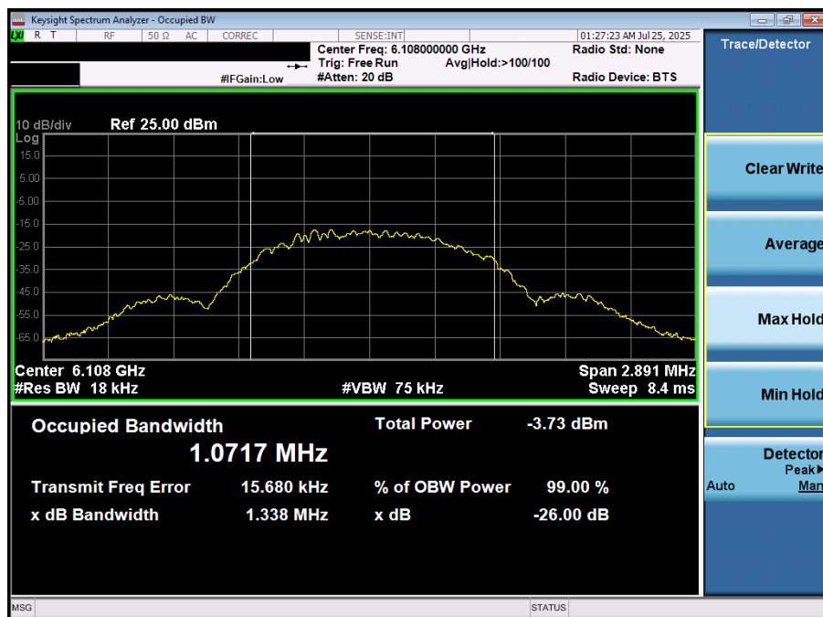
Plot 7-4. 26dB BW & 99% OBW (NB UNII LE1M – 6108MHz)
