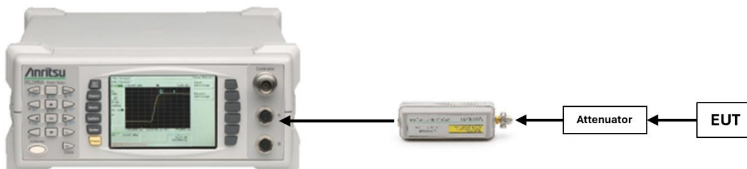
Figure 7-2. Test Instrument & Measurement Setup
