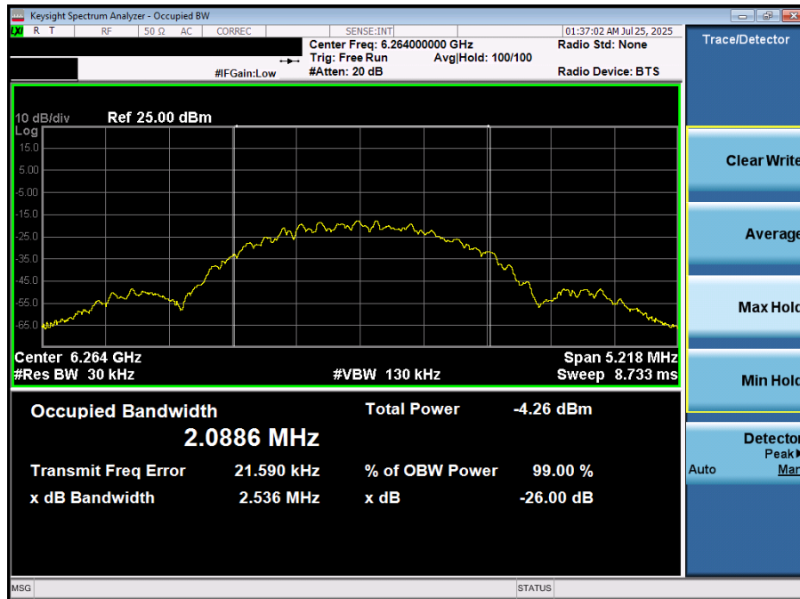
Plot 7-8. 26dB BW & 99% OBW (NB UNII LE2M – 6264MHz)
