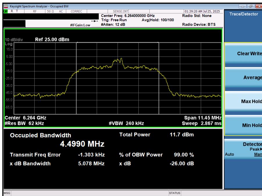
Plot 7-14. 26dB BW & 99% OBW (NB UNII HDR8 – 6264MHz)
