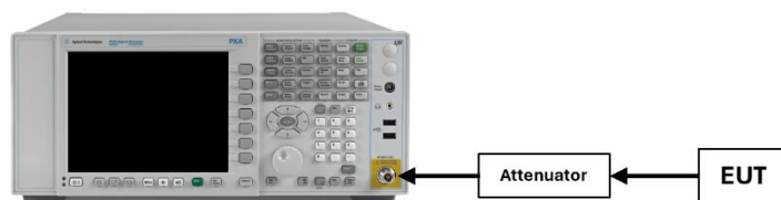
Figure 7-3. Test Instrument & Measurement Setup
