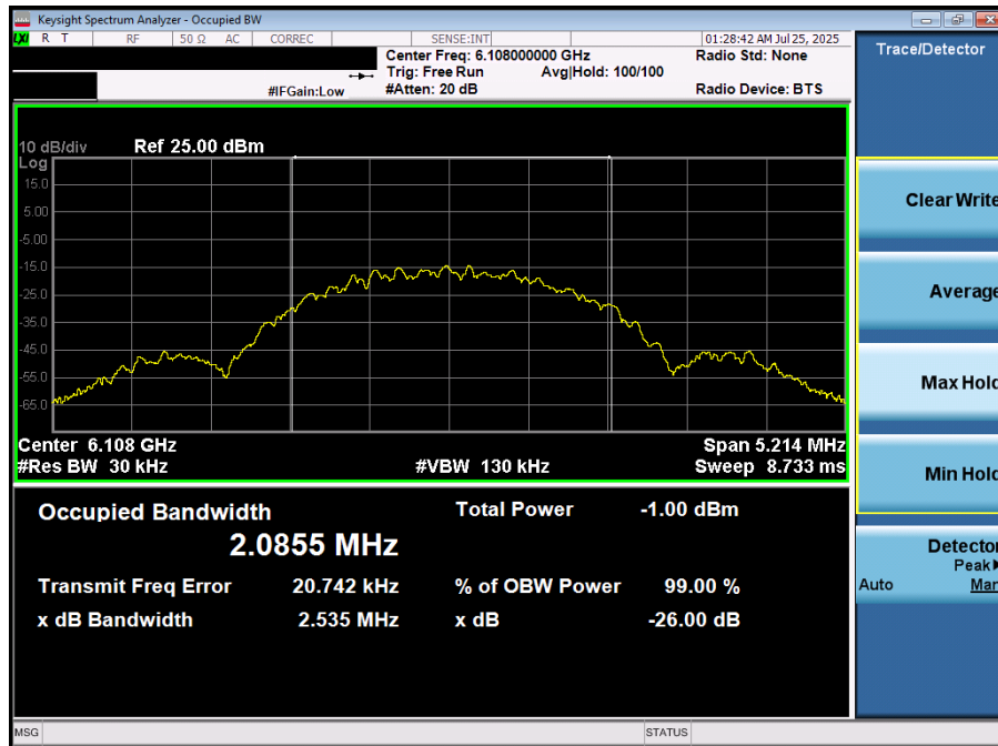
Plot 7-7. 26dB BW & 99% OBW (NB UNII LE2M – 6108MHz)
