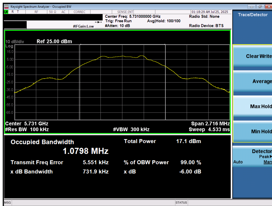
Plot 7-25. 6dB BW & 99% OBW (NB UNII LE1M – 5731MHz)
