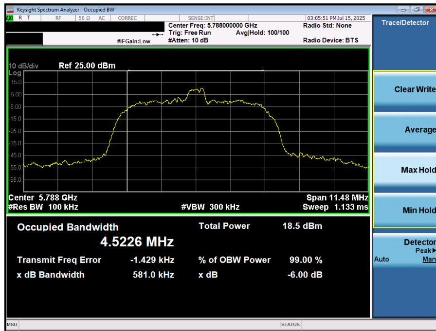
Plot 7-35. 6dB BW & 99% OBW (NB UNII HDR8 – 5788MHz)
