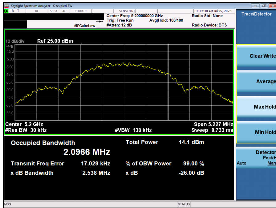
Plot 7-8. 26dB BW & 99% OBW (NB UNII LE2M – 5200MHz)
