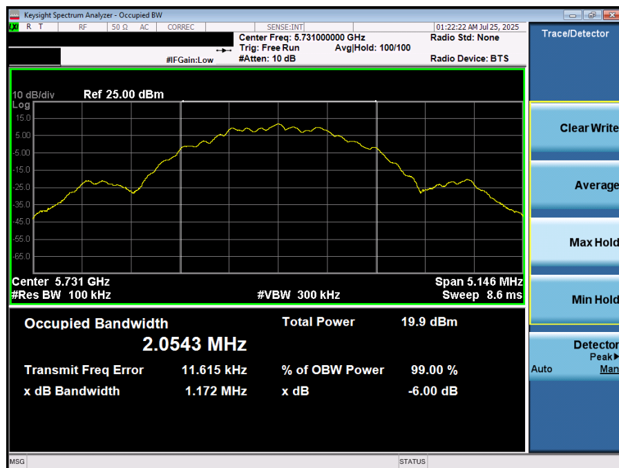
Plot 7-28. 6dB BW & 99% OBW (NB UNII LE2M – 5731MHz)
