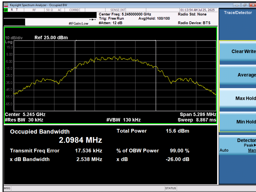
Plot 7-9. 26dB BW & 99% OBW (NB UNII LE2M – 5245MHz)
