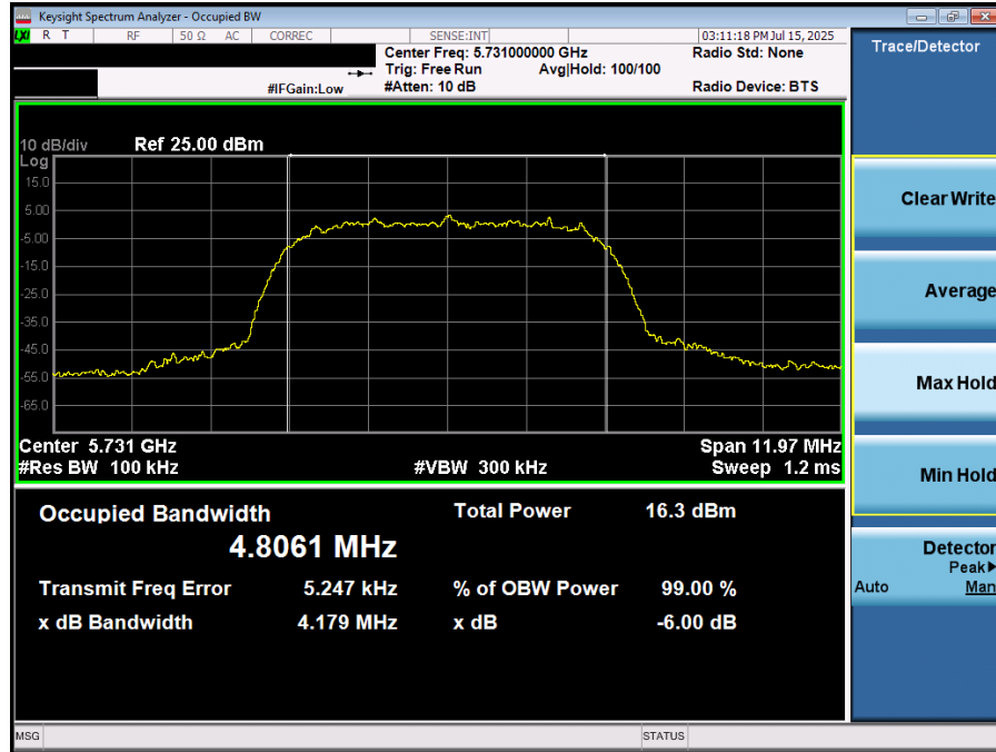
Plot 7-40. 6dB BW & 99% OBW (NB UNII HDRp8 – 5731MHz)
