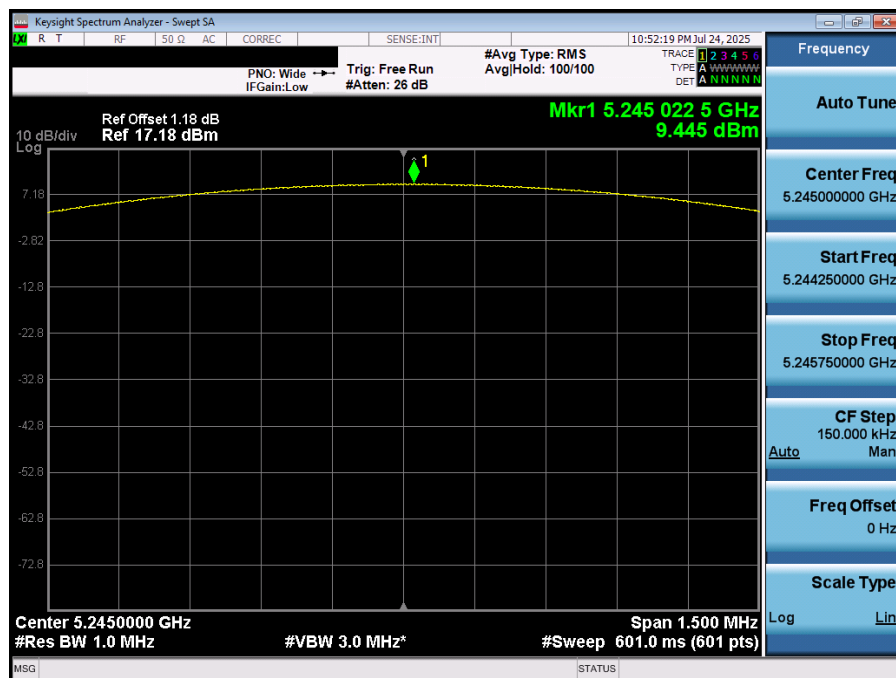
Plot 7-45. PSD (NB UNII BDR – 5245MHz)
