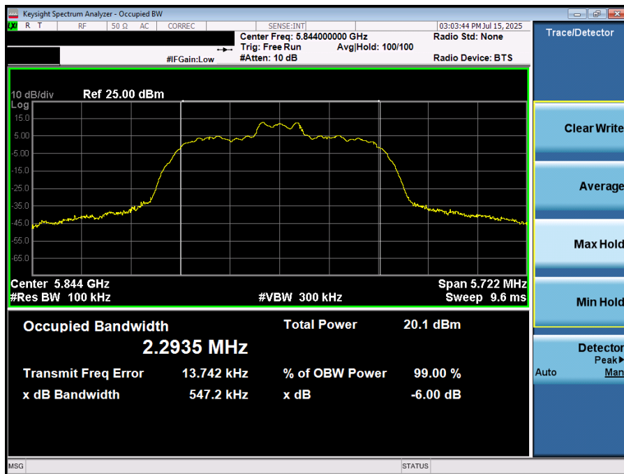
Plot 7-33. 6dB BW & 99% OBW (NB UNII HDR4 – 5844MHz)
