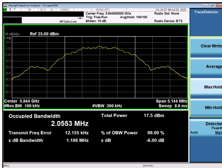
Plot 7-30. 6dB BW & 99% OBW (NB UNII LE2M – 5844MHz)
