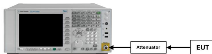
Figure 7-2. Test Instrument & Measurement Setup
