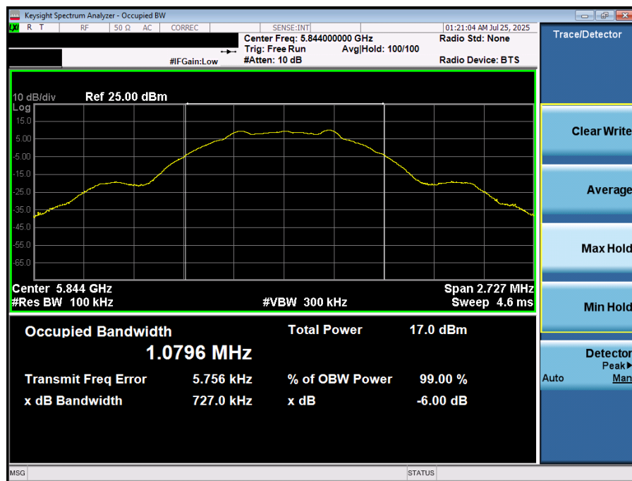
Plot 7-27. 6dB BW & 99% OBW (NB UNII LE1M – 5844MHz)
