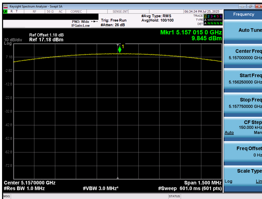
Plot 7-43. PSD (NB UNII BDR – 5157MHz)
