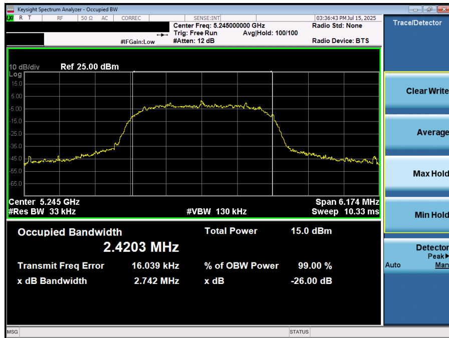
Plot 7-18. 26dB BW & 99% OBW (NB UNII HDRp4– 5245MHz)
