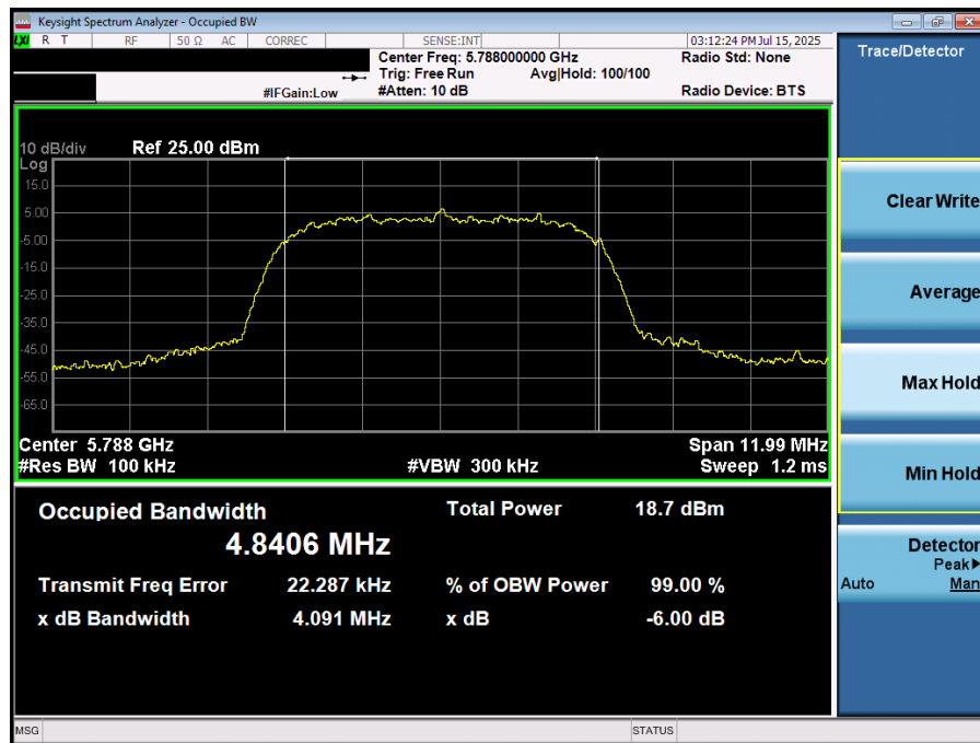
Plot 7-41. 6dB BW & 99% OBW (NB UNII HDRp8 – 5788MHz)
