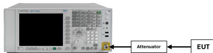
Figure 7-1. Test Instrument & Measurement Setup
