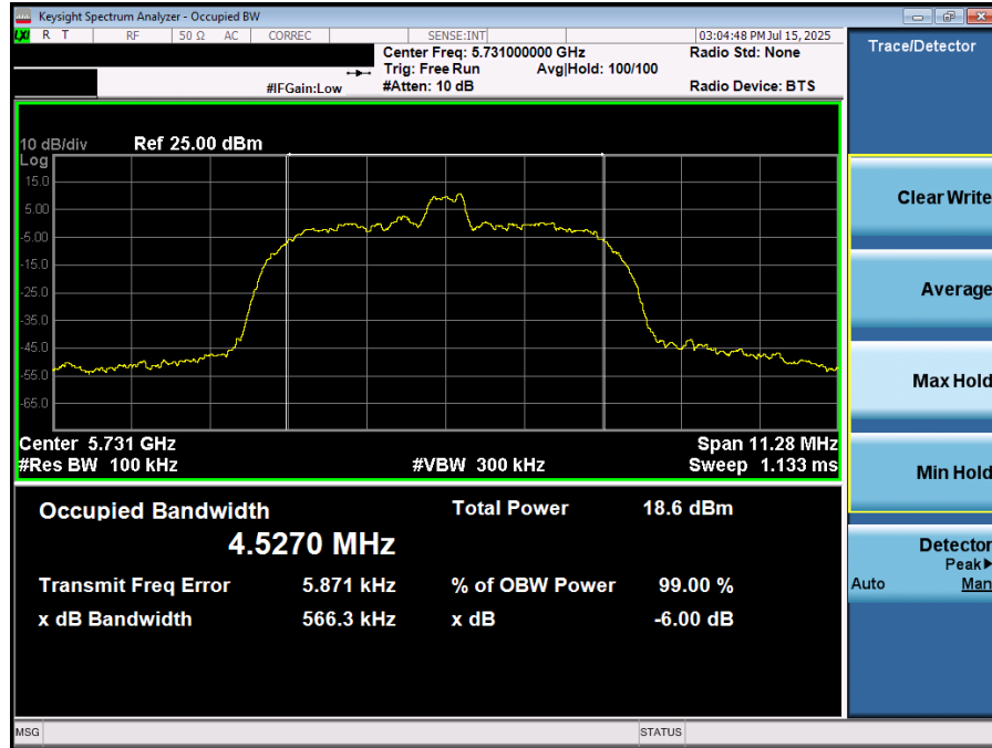
Plot 7-34. 6dB BW & 99% OBW (NB UNII HDR8 – 5731MHz)
