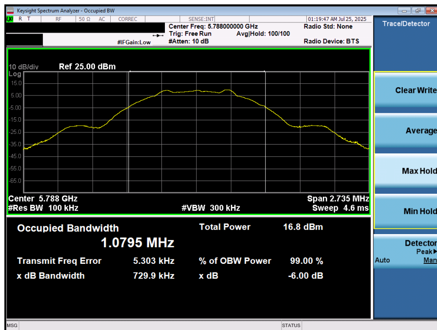
Plot 7-26. 6dB BW & 99% OBW (NB UNII LE1M – 5788MHz)
