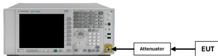
Figure 7-5. Test Instrument & Measurement Setup
