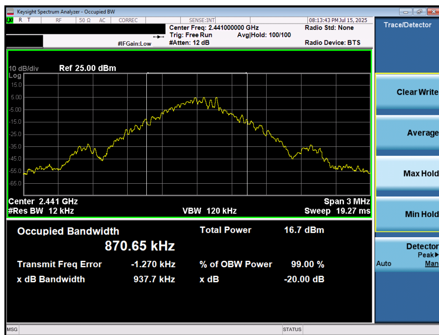
Plot 7-2. 20dB BW and 99% OBW Plot (Bluetooth, GFSK – Ch. 39)
