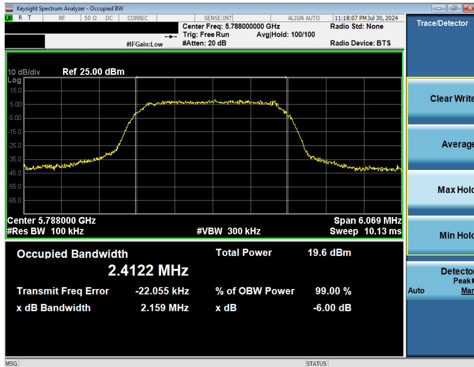
Plot 7-32. 6dB BW & 99% OBW (NB UNII HDRp4 – 5788MHz)
