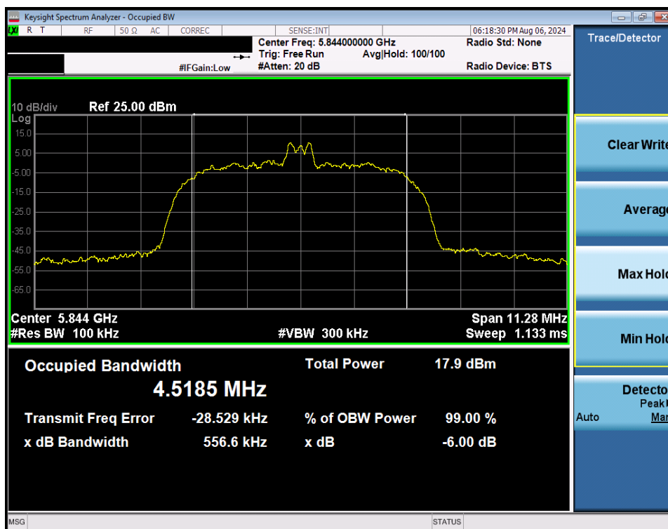
Plot 7-30. 6dB BW & 99% OBW (NB UNII HDR8 – 5844MHz)
