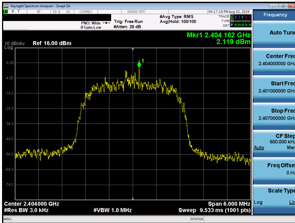
Plot 7-13. Power Spectral Density Plot (Bluetooth (HDR4), 4Mbps, – Ch. 1)
