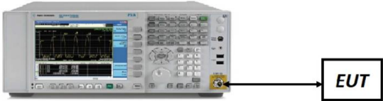
Figure 7-1. Test Instrument & Measurement Setup
