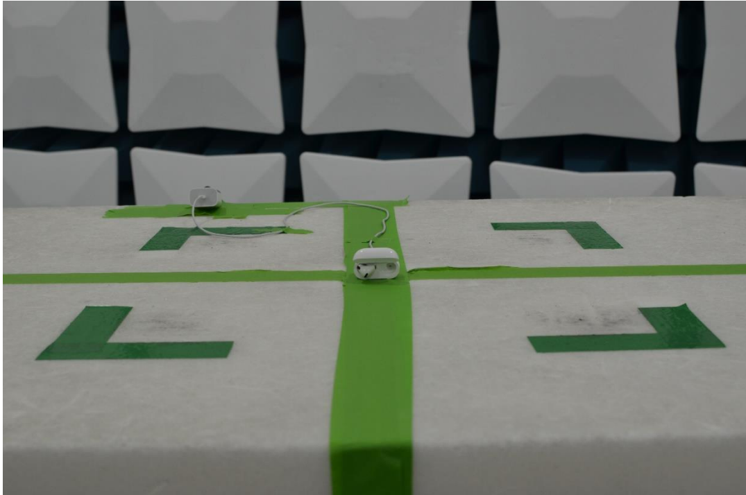
Figure 11: 30MHz-1GHz Test Setup (Front View)
