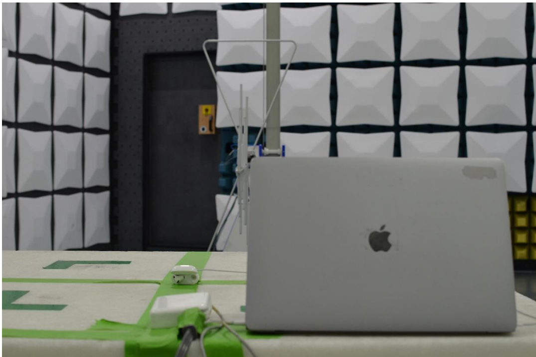
Figure 18: 30MHz-1GHz Test Setup (Rear View)
