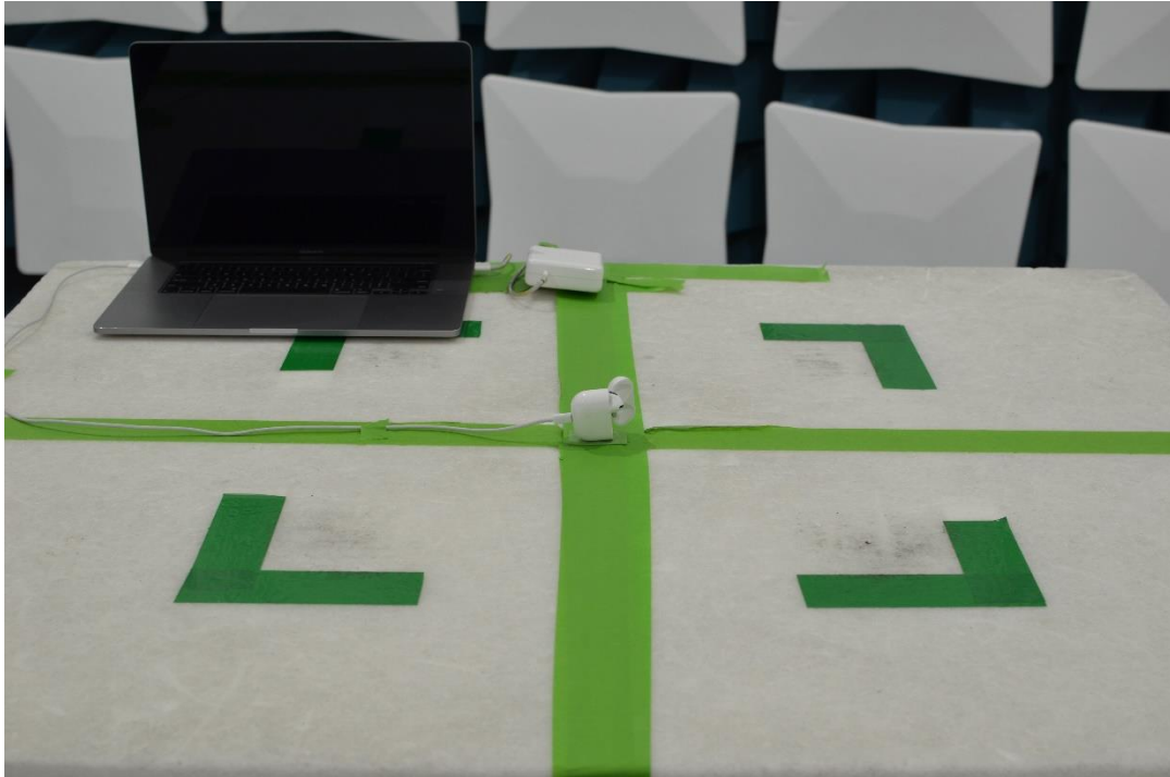
Figure 19: 30MHz-1GHz Test Setup (Front View)
