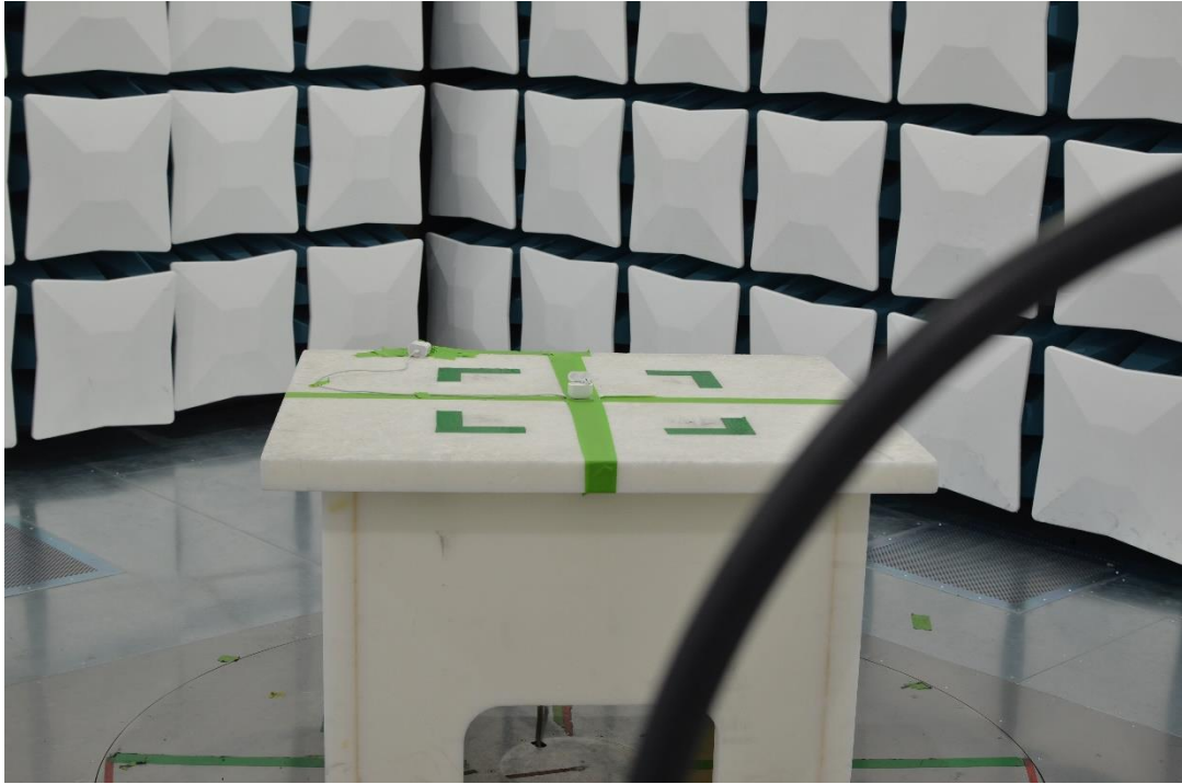
Figure 25: 9kHz-30MHz Test Setup (Front View)
