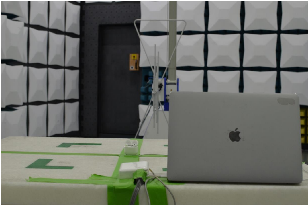
Figure 22: 30MHz-1GHz Test Setup (Rear View)
