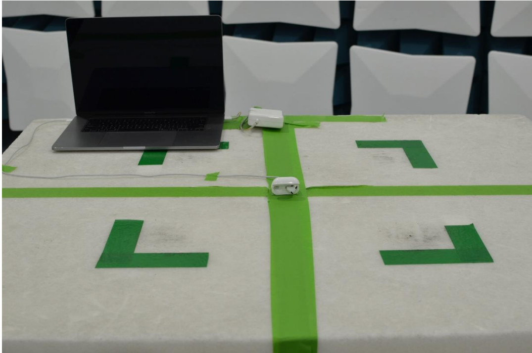
Figure 17: 30MHz-1GHz Test Setup (Front View)
