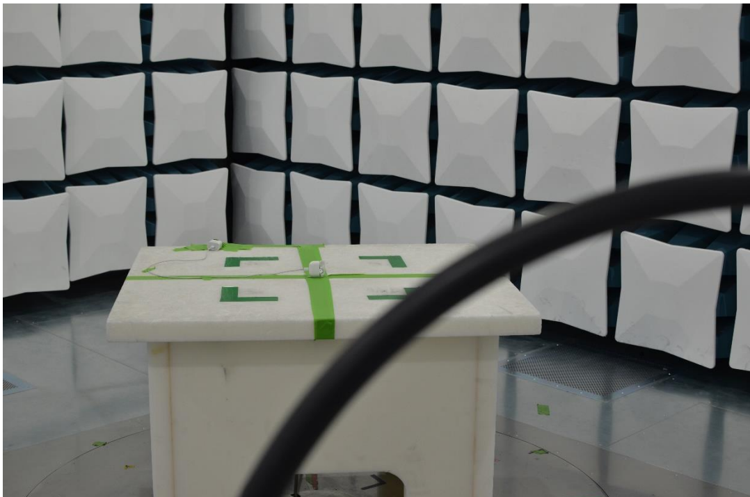
Figure 24: 9kHz-30MHz Test Setup (Front View)
