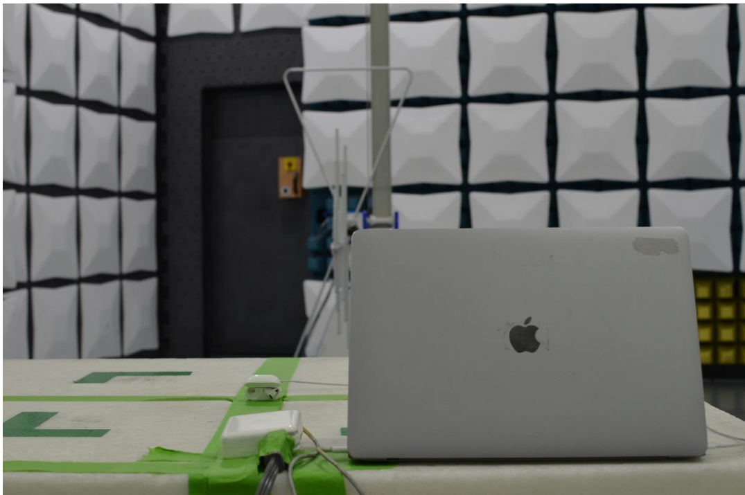
Figure 18: 30MHz-1GHz Test Setup (Rear View)
