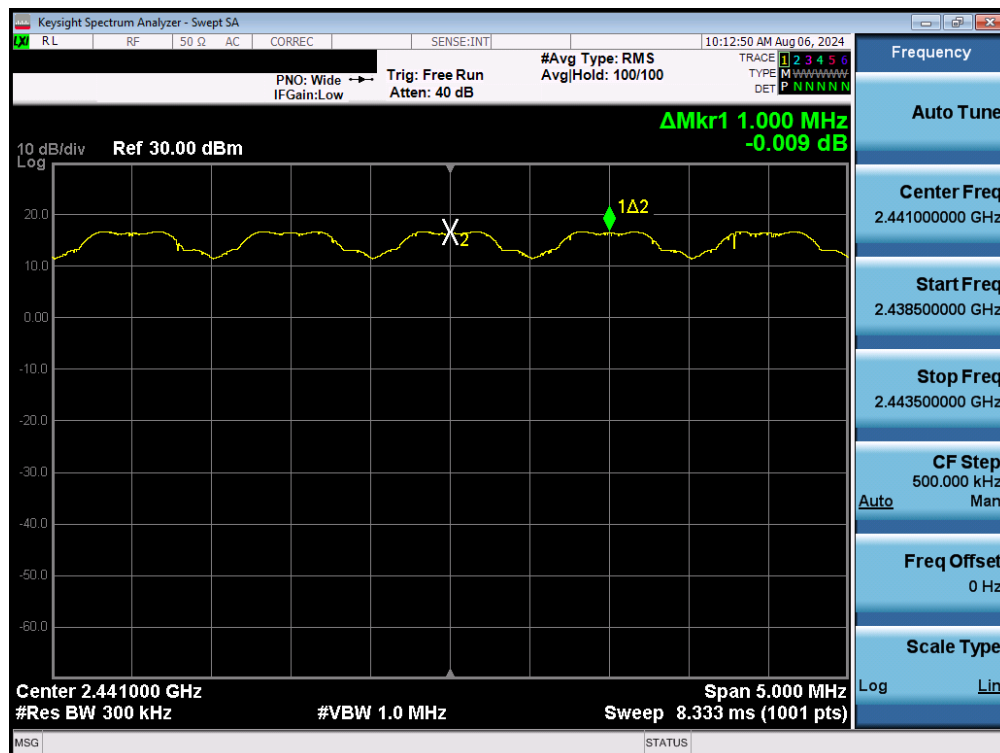
Plot 7-16. Channel Spacing Plot (Bluetooth, 8DPSK)
