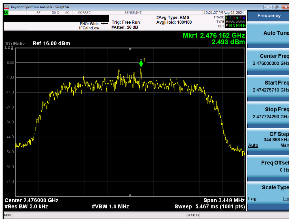
Plot 7-15. Power Spectral Density Plot (Bluetooth (HDR4), 4Mbps, – Ch. 73)
